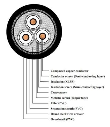
Figure 1: Cable construction as per IEC 60502-1 and BS 6622
